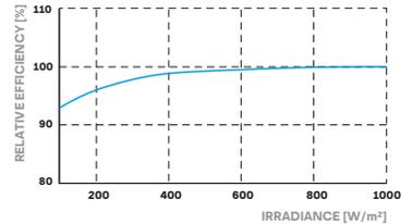
Typical module performance under low irradiance conditions in comparison to STC conditions (25 °C, 1000 W/m<sup>2</sup>)
